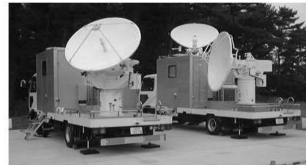
FIG. 1. Photograph of developed multiparameter radar system. X-band (right) and Ka/W-band (left) radar subsystems are mounted on 4-ton trucks. The antenna on the top of
