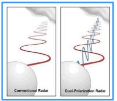
Working principle of a conventional (single, horizontal polarization) radar versus a dual polarization (horizontal and vertical) radar (Source: NOAA).
